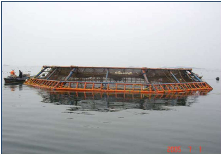
Fig. 20 PDW Submersible Fish Cage developed by Fishery Machinery and Instrument Research Institute (FMIRI°, Shanghai, China)
