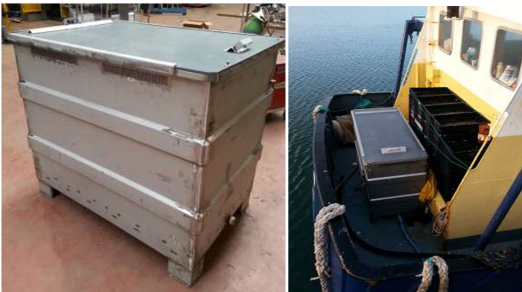
Fig. 23 Habitat tank for grey shrimp on board a shrimp fishing vessel (Photo: Xavier Vermeersch).
