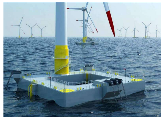
Ideol floating wind turbine acquired by Gaelectric, Ireland Floating offshore wind | BW Ideol (bw-ideol.com)
